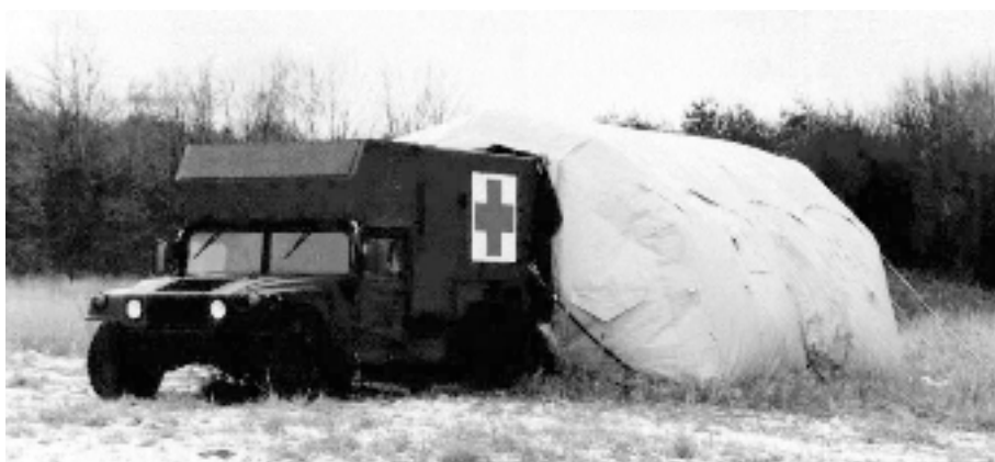
Figure J-10. Chemical Biological Protective Shelter (CBPS)
